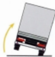
2 Factors such as load placement and shifting of weight will move the vertical down force at the wheels of the trailer
