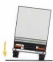
3 EB+ applies the trailer brakes to slow and stabilise the trailer
